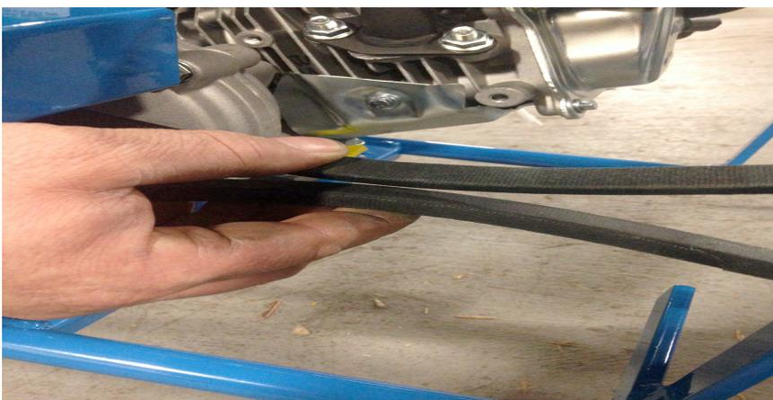
21. Attach the V-Belt by pushing it over belt guide bar, between the belt guard opening and then looping it over the engine drive pulley. See Figure 9.
