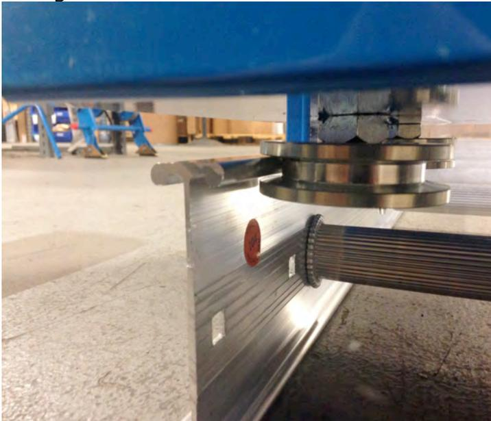
6. Slide the carriage along the track to base section so that the bumpers rest on the base section. Make sure carriage slides smoothly on track.
